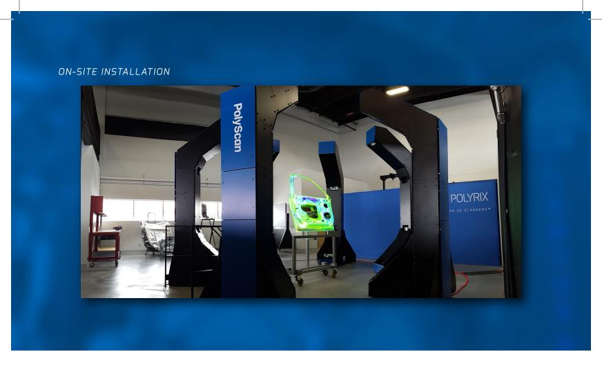
Our SURROUND 3D SCANNERS™ are by design immobile during the inspection. This makes them safe and simple to operate: place a part in the center and press Scan. Their unique calibration avoids the need for data alignment and their multiple baselines increase accuracy when measuring points.
