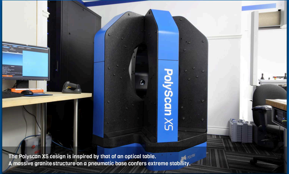
The PolyScan XS combines 24 scanning units: 12 cameras and 12 projectors linked together.
